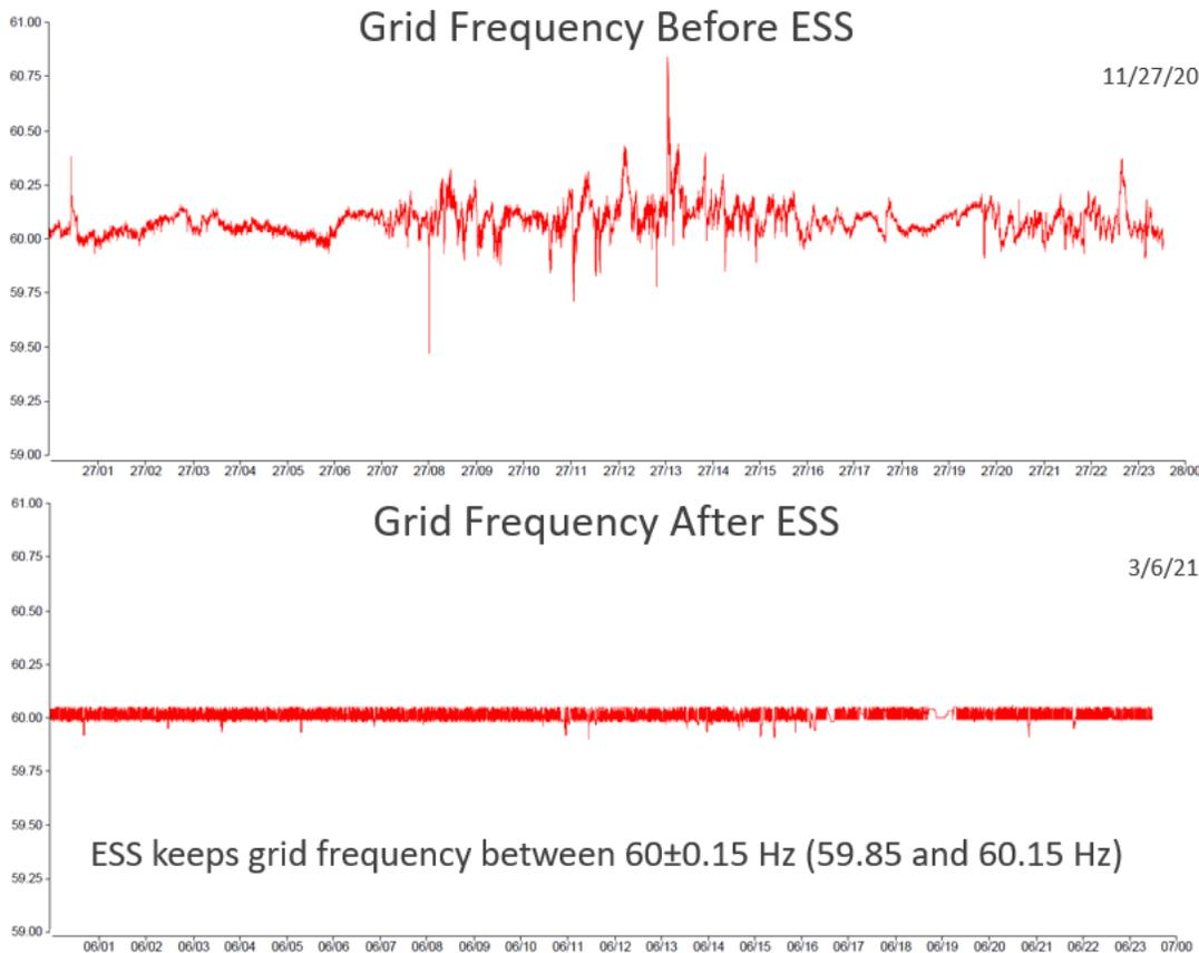
The 40 MW ESS system became fully operational on March 1, 2021. The system will eliminate more than 70% of short duration outage due to generator and renewable intermittency trips.
